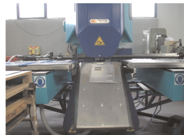
Components are punched and either microtagged or automatically unloaded
